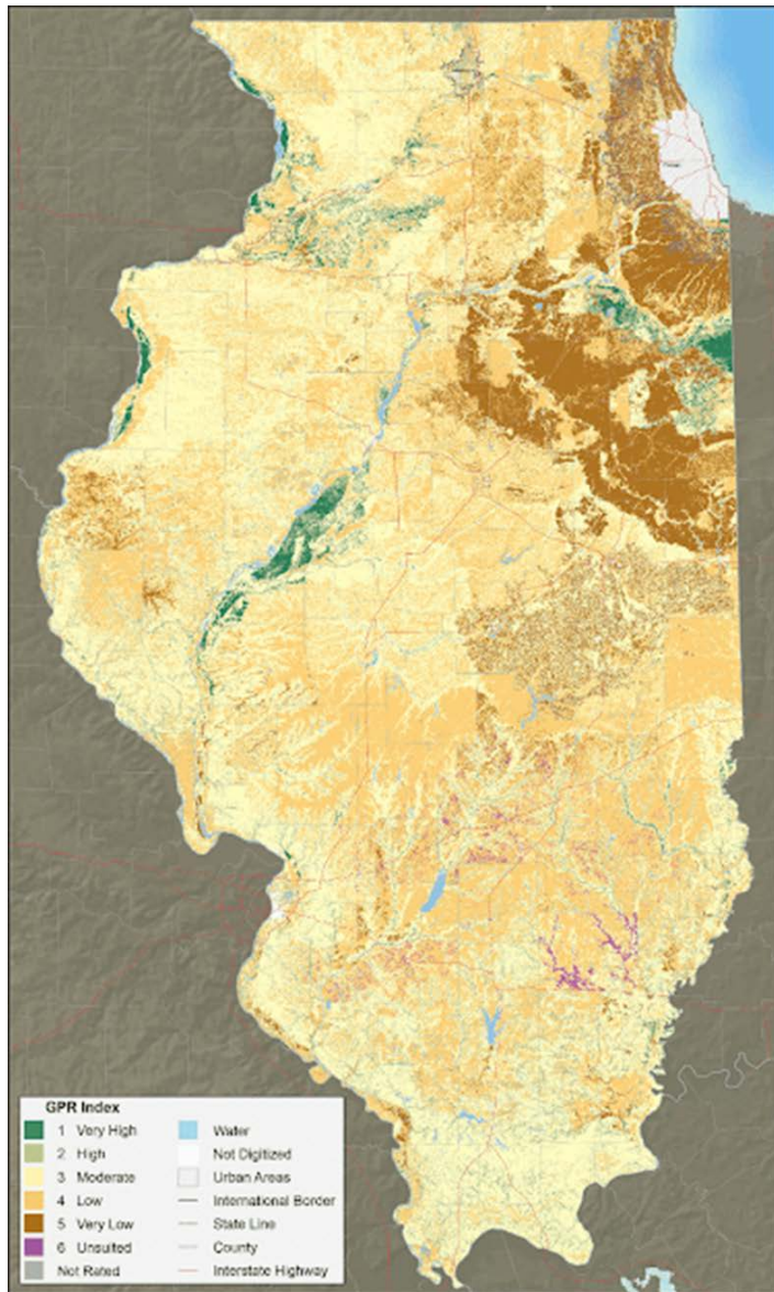
Figure 10 – GPR Soil Suitability Map for Illinois. Very Low GPR Index for the project area. Poor likelihood of satisfactory results is prevalent in this area
